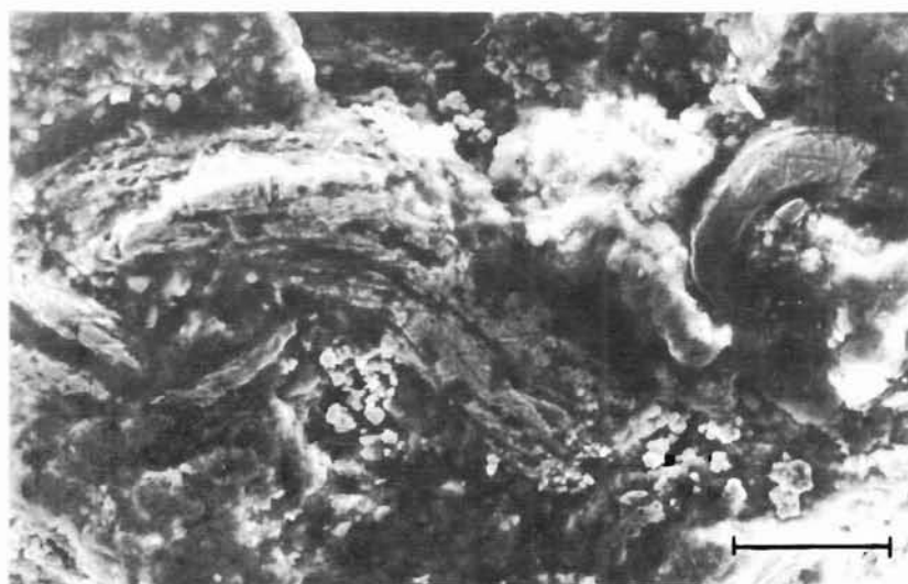
FIGURE 6. Filiform native silver crystals on nickeline with annabergite. Backscattered electron image. Scale bar 0.02 mm.
